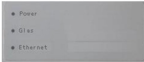
Figure 3-2 LED Indicators of ZTE ZXHN F3100
